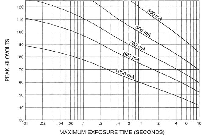
Nominal anode input power for the anode heat content 40%. IEC 60613
