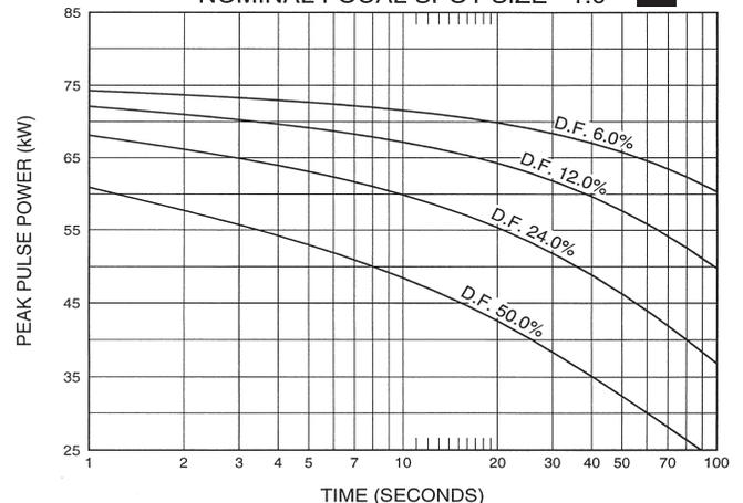
Nominal anode input power for the anode heat content 70%. IEC 60613
