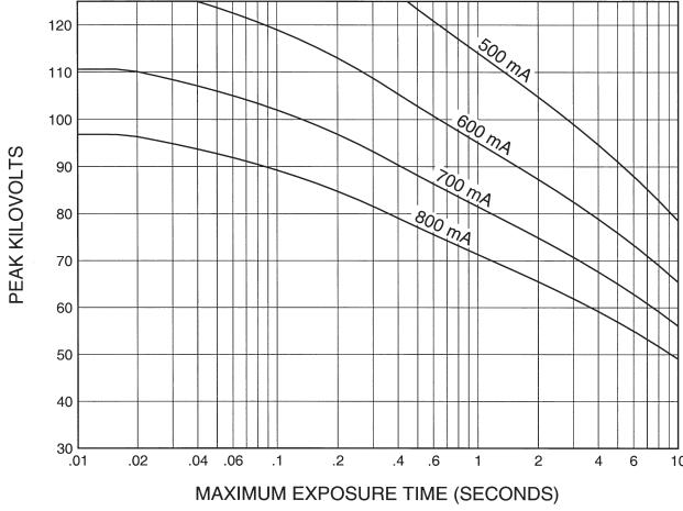
Nominal anode input power for the anode heat content 40%. IEC 60613
