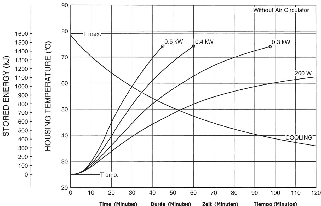
**Operating Temperature:** Minimum ambient temperature for storage and transportation is -20°C (0°F). Operating range of the ORIII housing is 16° - 72°C (60° - 167°F).
