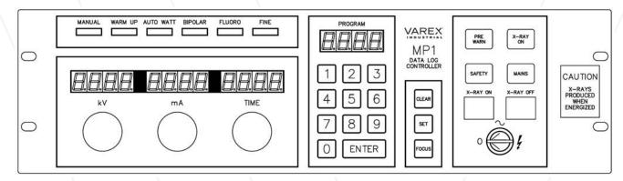
19 inch Rack Mount: Width 482mm (19.6") Height 133mm (5.4") Depth 240mm (9.75") Weight 3.5 Kg
