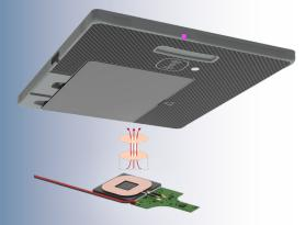
WIRELESS CHARGING Allows charging to be incorporated into accessories such as a bucky or a carry case so that a battery might never be removed
