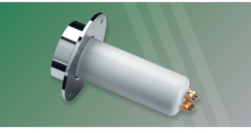
The CA7-type receptacle socket has 4 symmetrically positoned pins standard for X-ray cable plugs and receptacles. It complies to NEMA XR-7 and IEC60526.
