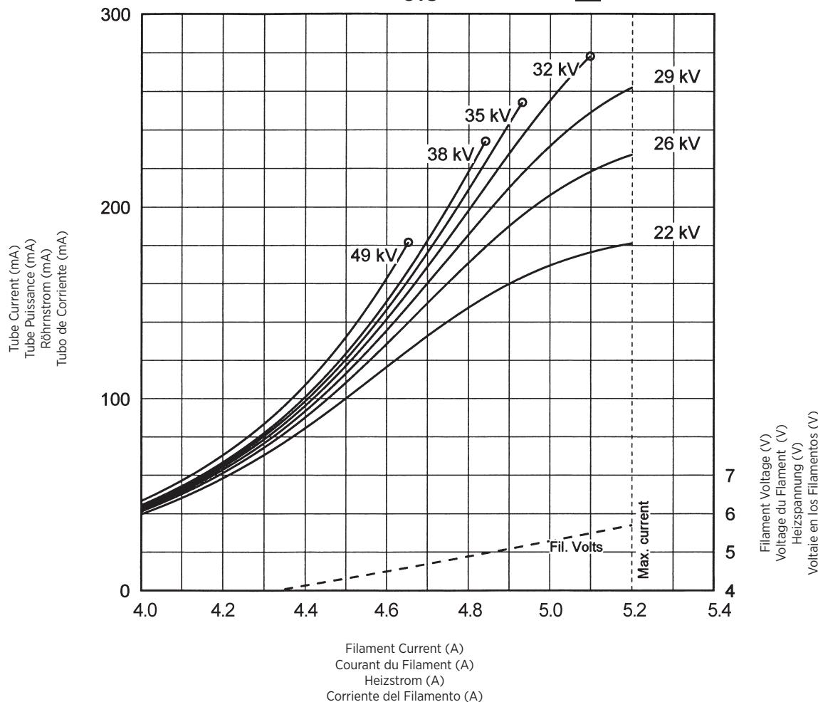
Note: When using these emission curves for trial exposures, refer to the power rating curves shown for maximum kV, tube emission, filament current, exposure time, and target speed.
