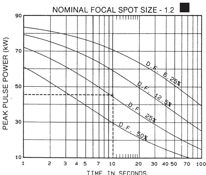
Nominal anode input power for the anode heat content 70%. IEC 60613
