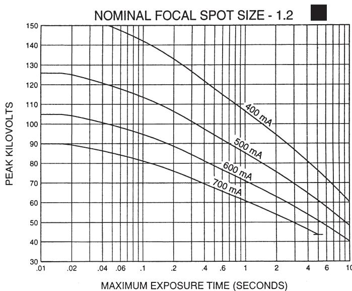
Nominal anode input power for the anode heat content 40%. IEC 60613
