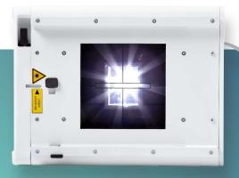
Beam filtration is possible with the optional motorized filter module. Choose between no filtration or three different aluminum plus copper combinations.
