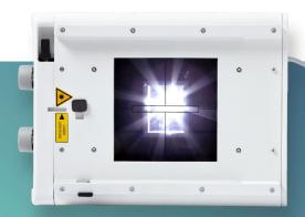
The beam filtration is possible with the optional motorized filter module. No filtration or three different aluminum plus copper combination filtrations are available. Shutter calibration and customization of user settings are easily performed through the software menu, accessible via the display.
