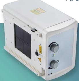
The beam filtration is possible with the motorized filter module. No filtration or three different aluminium plus copper combination filtrations are available.
