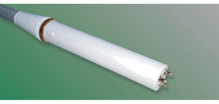
Varex Imaging CA16 high voltage cable assemblies are X-ray cables terminated with 3-pin (O3) Extended Federal Standard terminations rated up to 160 kVDC for medical and industrial applications. These assemblies are type tested under the severest life (aging) conditions.
