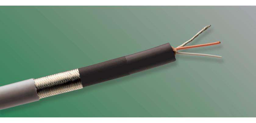
Highly flexible, small diameter, low capacitance, 3-conductor, 100 kVDC rated rubber insulated high voltage cable.
