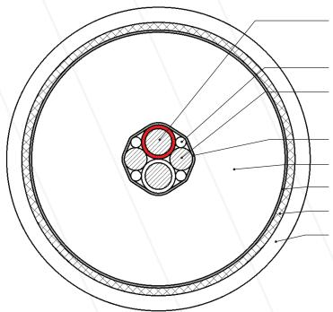
Red and white ETFE insulated conductors,  $1.8 \text{mm}^2$  (19 x Ø0.35 mm), stranded tinned copper wires.
