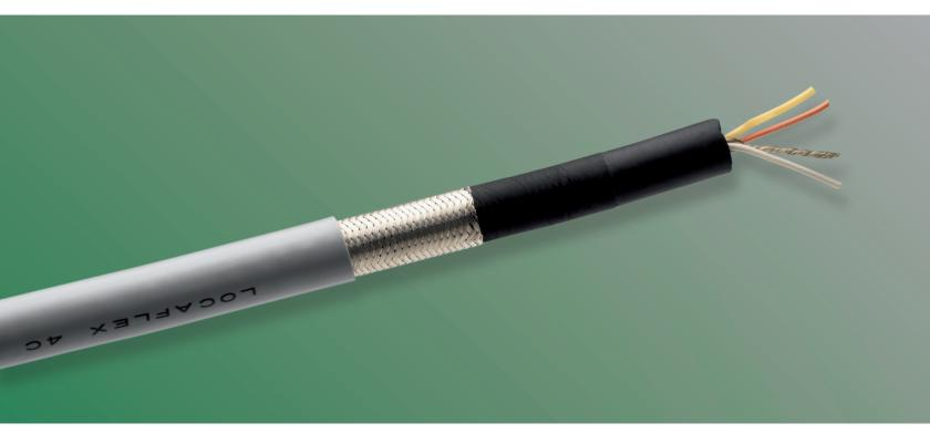
Highly flexible, small diameter, low capacitance, 4-conductor, 75 kVDC rated rubber insulated high voltage cable.
