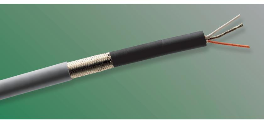
Highly flexible, small diameter, low capacitance, 3-conductor, 75 kVDC rated rubber insulated high voltage cable.
