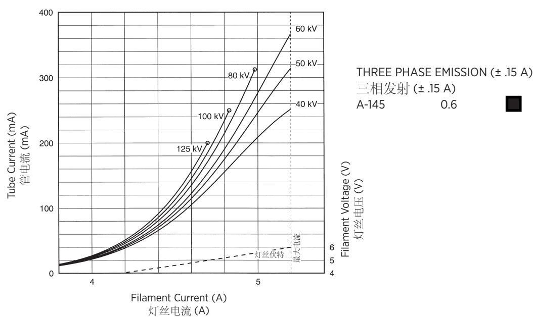
Note: When using these emission curves for trial exposures, refer to the power rating curves shown for maximum kV, tube emission, filament current, exposure time, and target speed.
